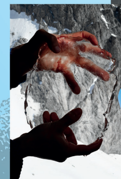
ice after being extracted from the glacier and cutted with a saw into a ± 3 cm sheet
