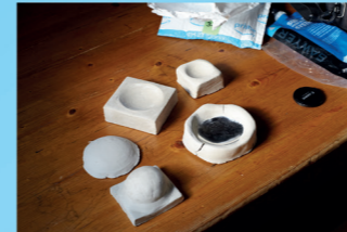
First molds are made with clay. Then 3D printed. Another version uses CNC to create a metal mold that can be heated up, accelerating the process of lens making.
